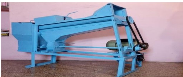
Fig. 1. Actual fabricated model of corn peeling and cutter machine.
